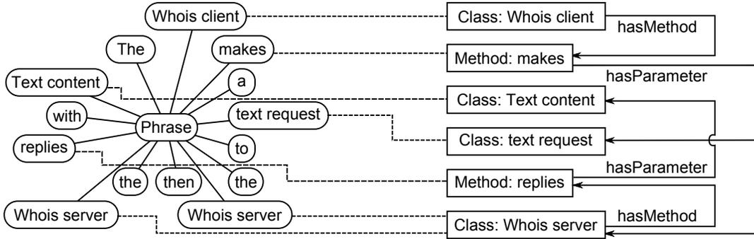
Figure 1. Tracking Edges Connect the Textual Nodes With their UML Counterparts.
