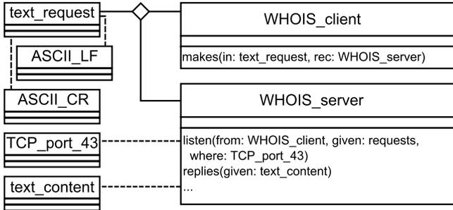
Figure 2. An Excerpt of the Generated UML Class Diagram for the WHOIS Protocol Specification.
