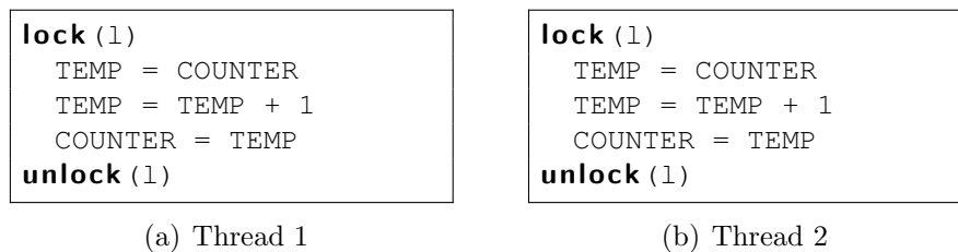
Figure 3.2.: Avoiding an atomicity violation by protecting the critical section with locks.
