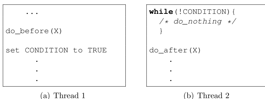
Figure 7.4.: Spinning read loop pattern.
