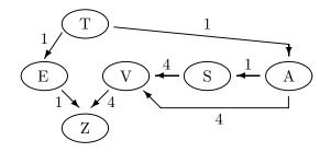
The number at the arrow between two components x and y in the diagram is the number of interfaces provided by y which are used by x. From the number of interfaces, the probability that a problem with a particular component (say, V) causes rework in a particular set of components (say, V, S, and A) can be computed (41.4 percent in the example).
