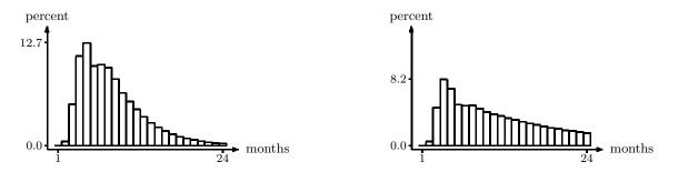
The chart to the left corresponds to minimal coupling, the chart to the right to maximal coupling. The expected values for the development time are 8.6 months for the first project and 13.5 months for the second. In the model, the stronger coupling thus leads to a more than fifty percent higher estimate for the second project. Minimal coupling will not occur in a "real world" design and maximal coupling should not, but the example makes clear how strong the impact of the coupling can be.
