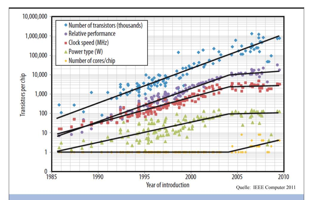
**Figure 1.** Transistors, frequency, power, performance, and processor cores over time. The original Moore's law projection of increasing transistors per chip remains unabated even as performance has stalled.
